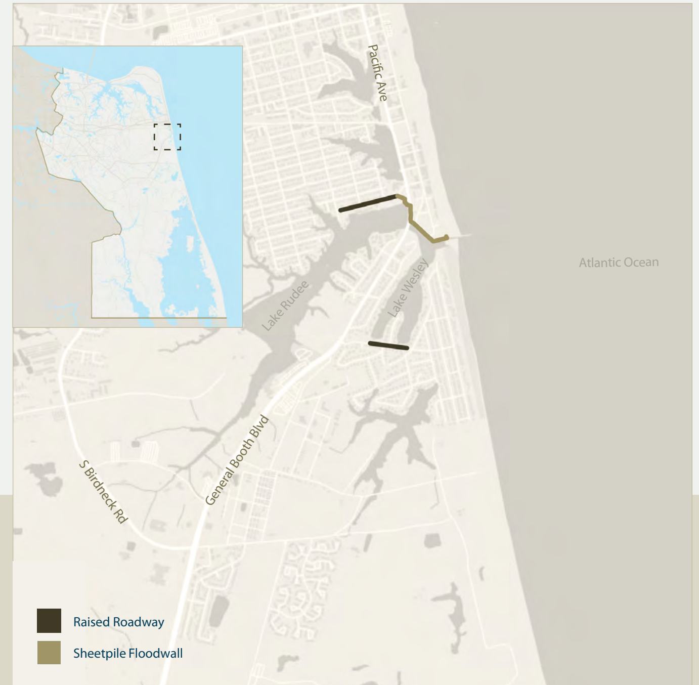
Rudee Heights alternative structural protection with raised roadway and floodwall
