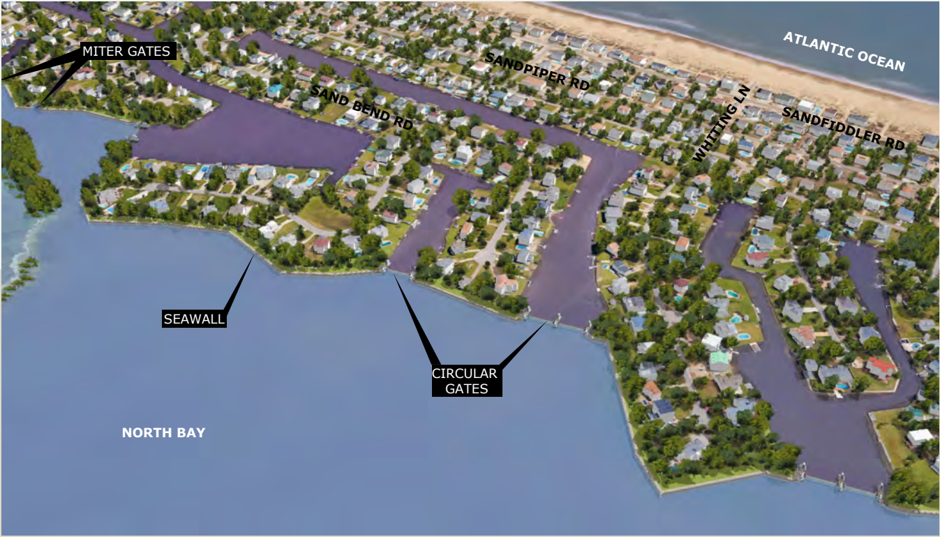
Sandbridge Neighborhood structural protection system under flood condition
