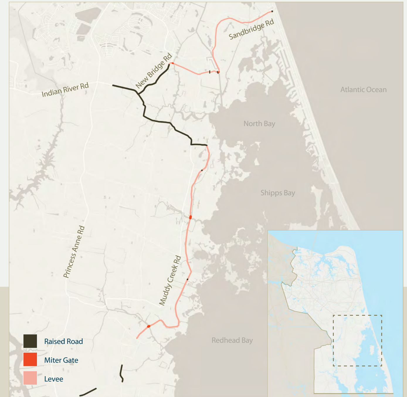
Sandbridge and Muddy Creek Road alternative alignment with raised roads, miter gates, and levees.
