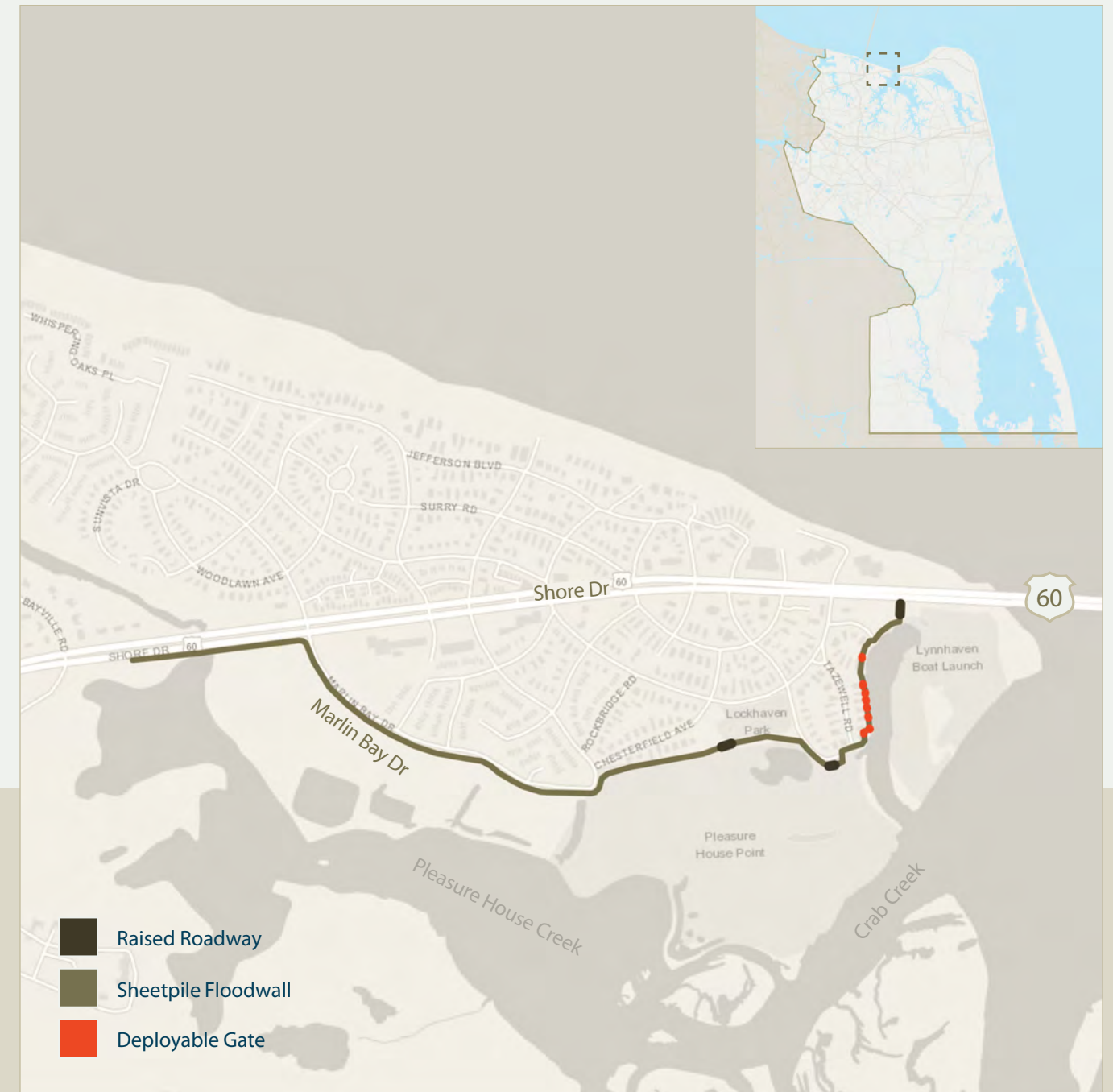
Location of West of Lesner Bridge structural protections with raised roadways, floodwalls, and deployable gates.
