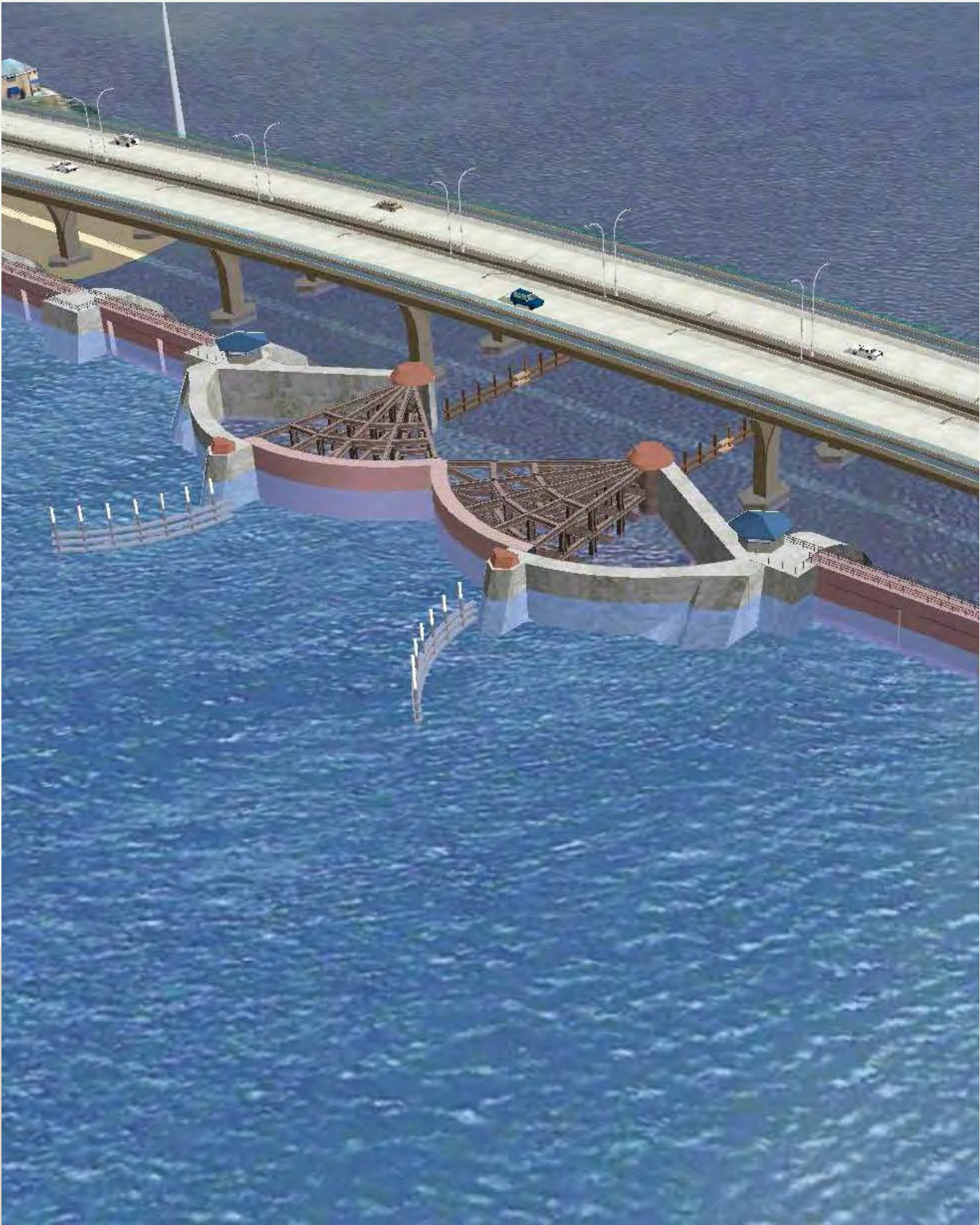
Lynnhaven Inlet circular and movable gate system under flood condition (enlarged view)
