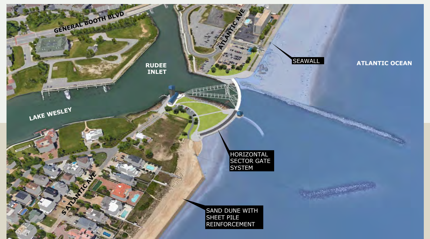
Rudee Inlet structural protection system under flood condition
