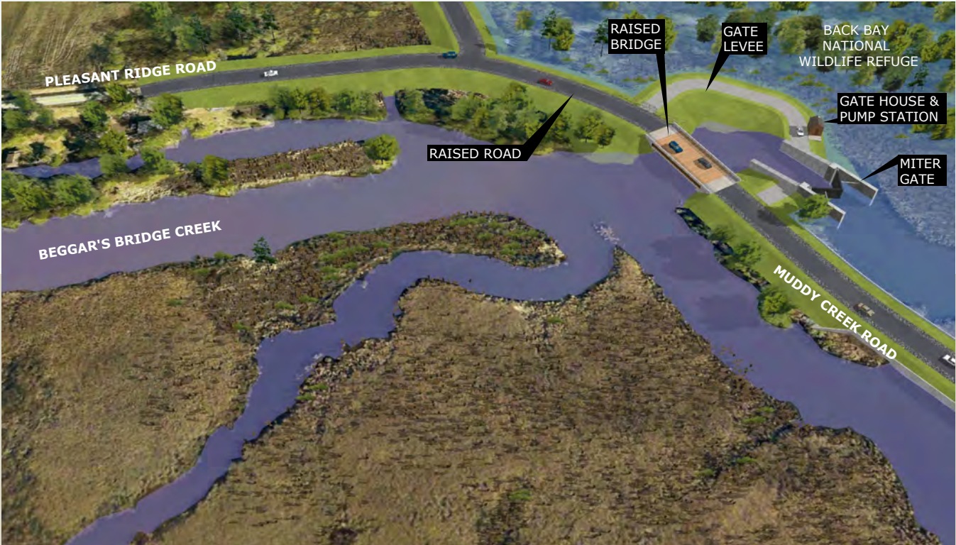
Muddy Creek Road structural protection system under flood condition
