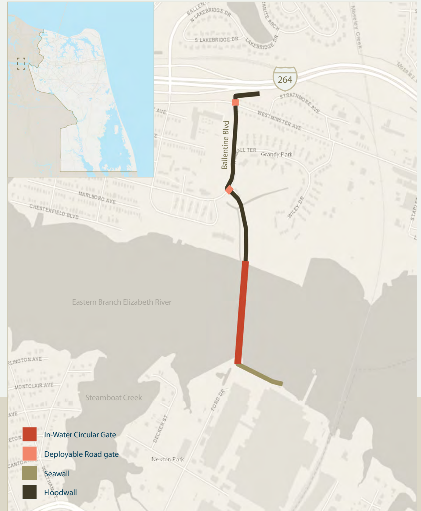
Elizabeth River alignment with circular gate, road gates, seawall, and floodwalls.
