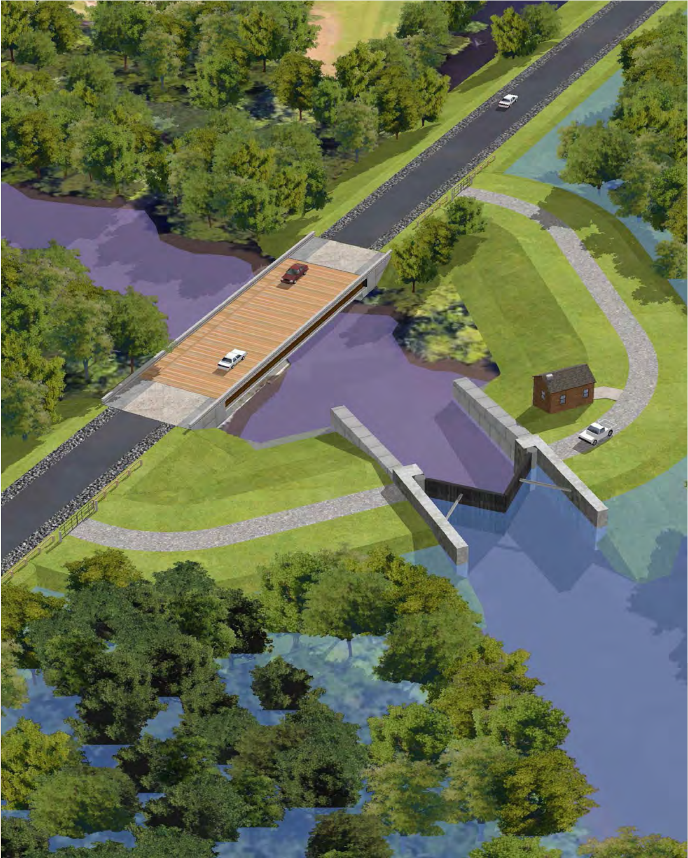
Sandbridge Road structural protection system under flood condition
