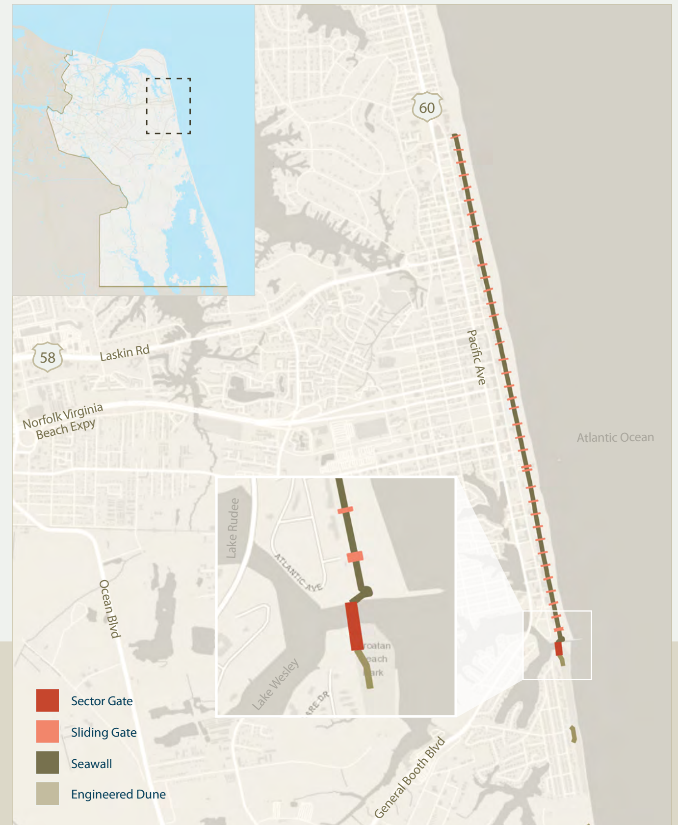
Atlantic Oceanfront alignment with seawalls, sliding gates, sector gate, and dunes.
